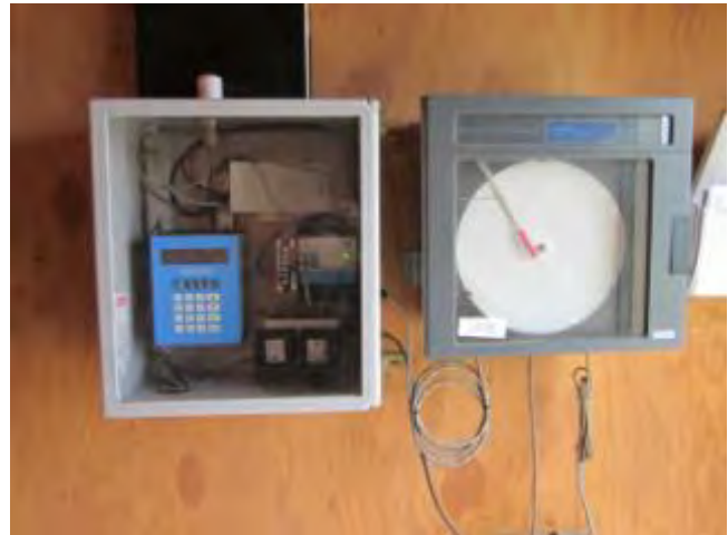
Meter inside the shack take continuous readings of the flow.
