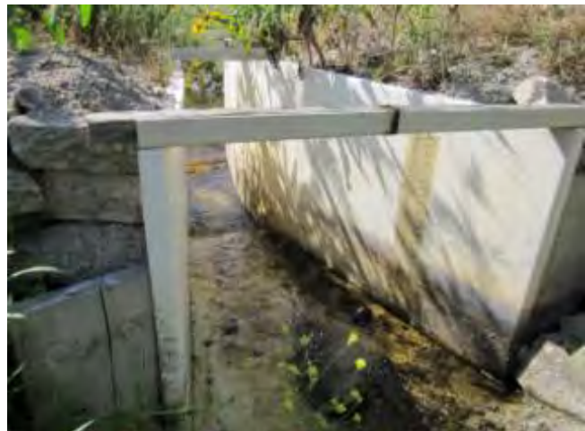
Parshall Flume just upstream from USGS Gauge.
