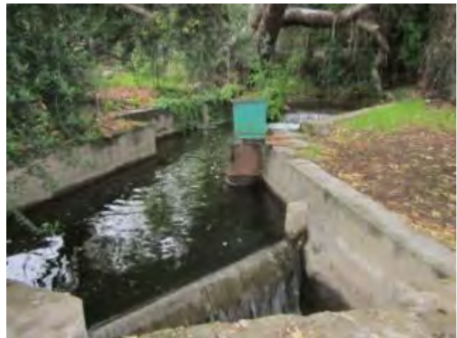
Green Box is a still well, Flow coming from Zanja.
