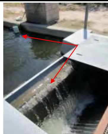
Northfork weir is measured with a weir and still well (red arrow).
