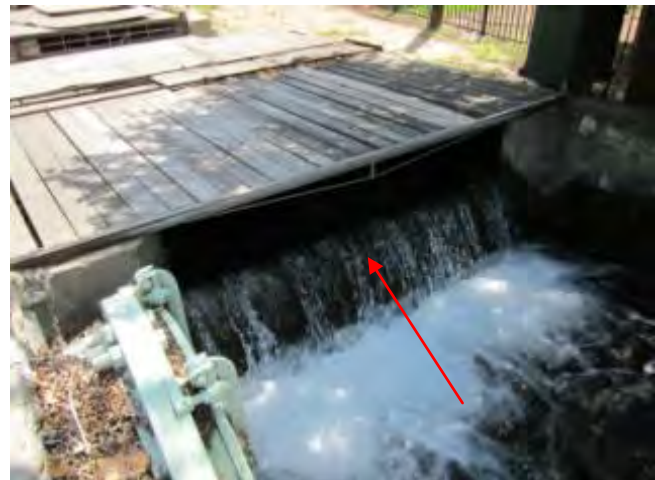
Flow is measured using a tape and weir (red arrow).
