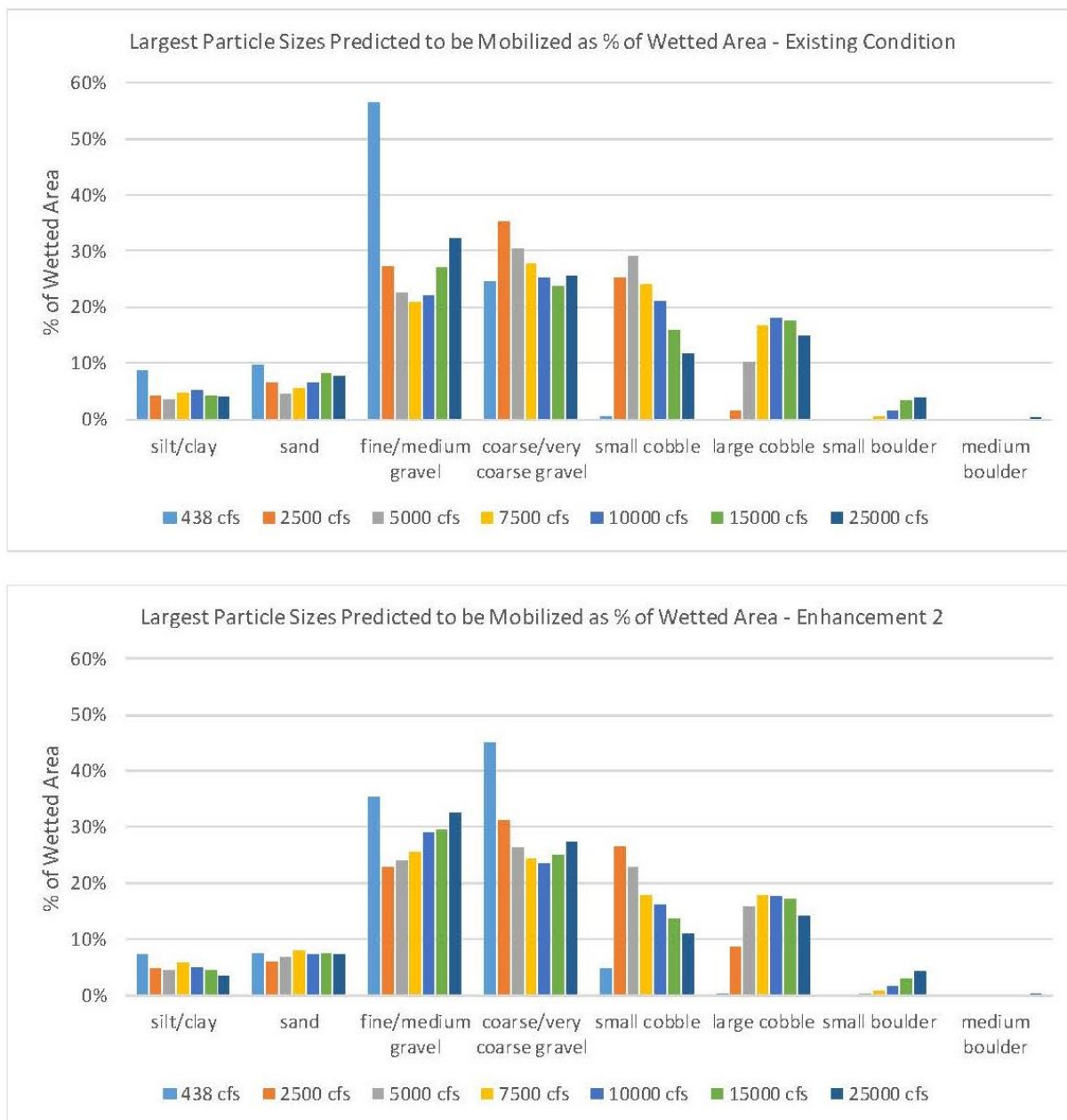
Figure 4-79. Percent of Flow Areas with Incipient Motion of Sediment Size Classes for Existing Condition (top) and with Enhancement 2 (bottom)
