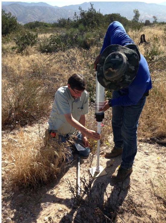
Figure 3. NHC and SBVWCD personnel preparing Constant Head Permeameter for percolation measurement
